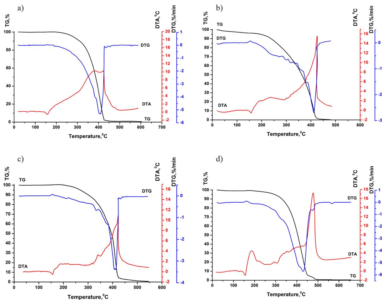
**Fig. 1.** Thermograms of the composites based on polypropylene and polyamide-6, previously modified with montmorillonite-polyvinylpyrrolidone mixture (MPM): a – sample 1 – PP, b – sample 2 – PP:(PA-6/MPM) = 95:5, c – sample 3 – PP:(PA-6/MPM) = 85:15, d – sample 4 – PP:(PA-6/MPM) = 70:30
