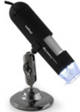
Fig. 8. USB microscope for quick visual evaluation
