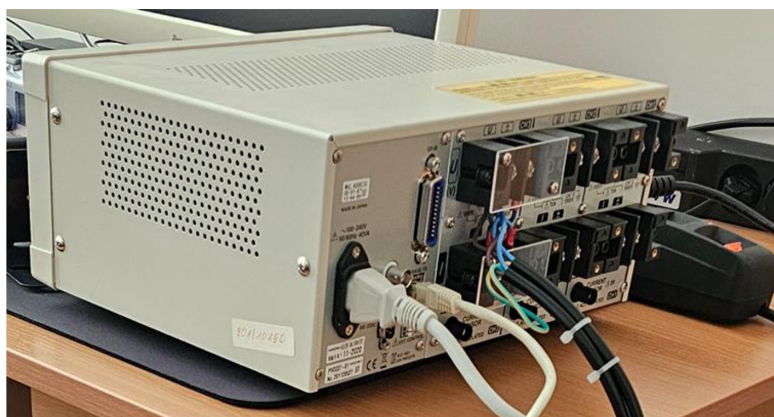
Figure 1. Connection of the HIOKI PW3337 to the measurement line
