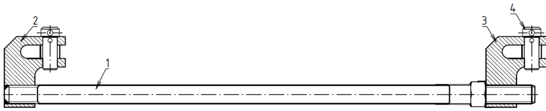
Figure 6. Adjustable coupling rod, straight type: 1) straight rod, 2) fixed bracket, 3) adjustable bracket, 4) adjustment pin
