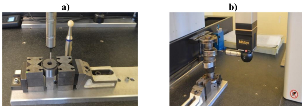
Figure 2. View during scanning of the geometry of the delivery valve a) and a fragment of the camshaft b)
