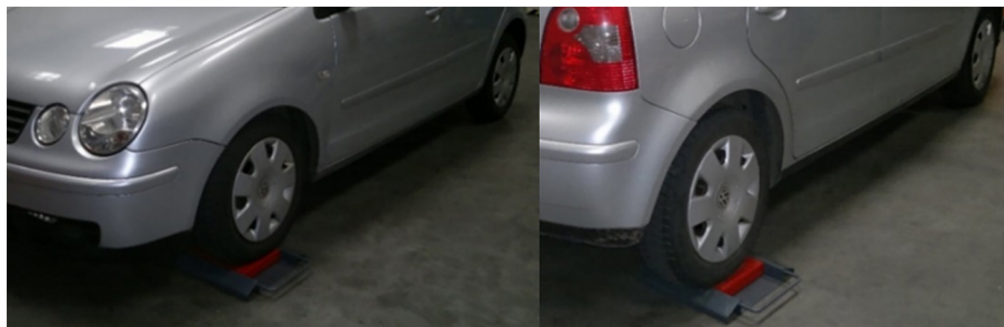
Figure 3. Plates allowing additional loads to be applied to the bodywork
