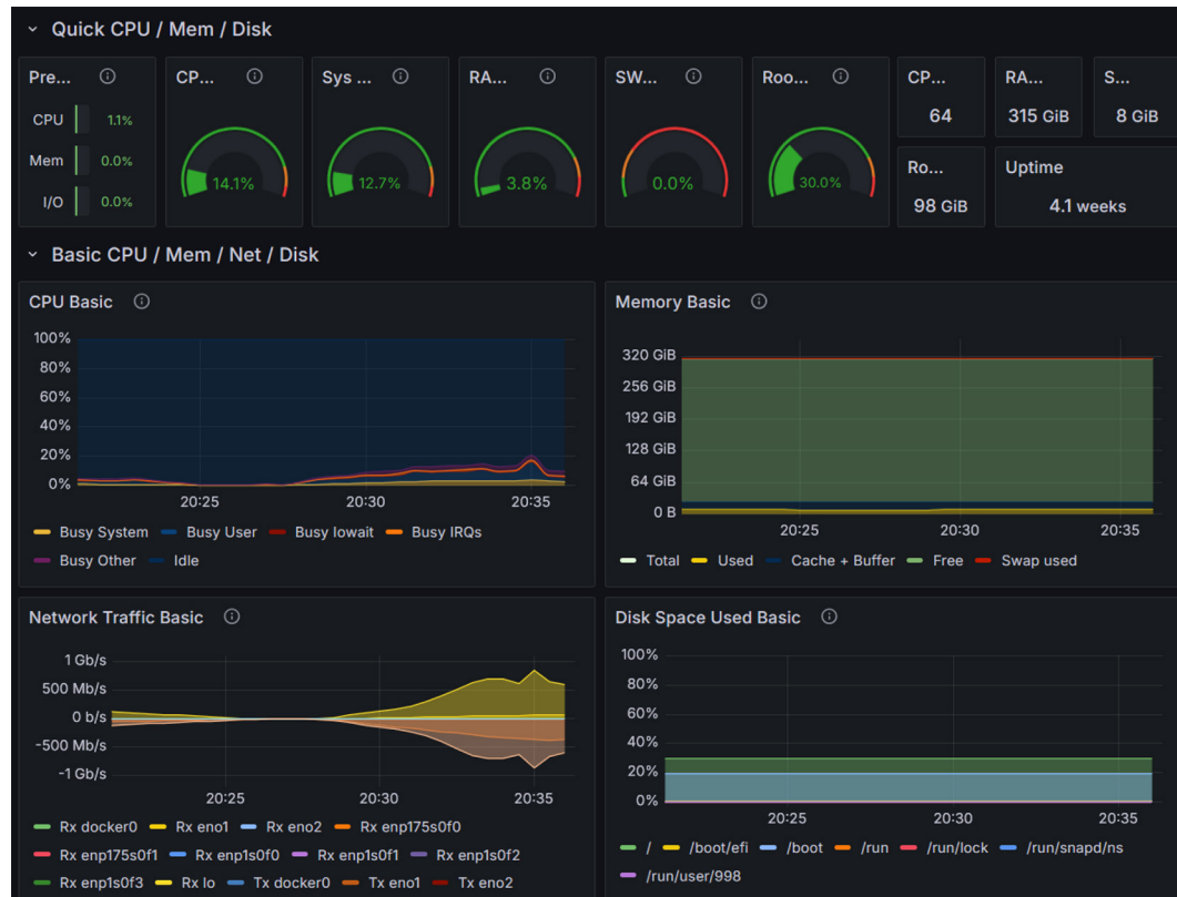
Figure 3. Server telemetry data at peak load, illustrating low CPU and memory consumption relative to total capacity, alongside a significant surge in network throughput on the external interface (above 400 client connections)
