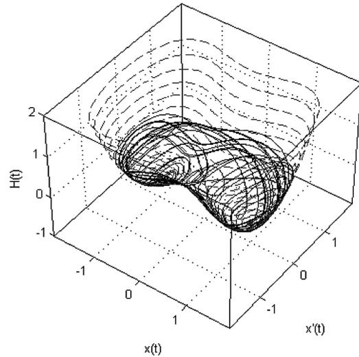
Fig. 3. Phase trajectories projection on the Hamiltonian surface in the case of chaotic state
