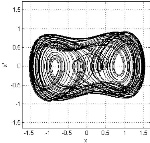
Fig. 1. Typical phase trajectories in chaotic state
