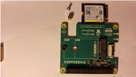
Figure 2. Raspberry Pi 5 with the NVMe M.2 HAT expansion board
