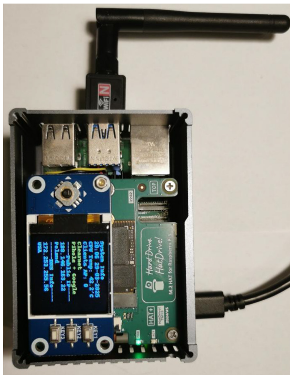
Figure 1. The TOR router assembly with a USB Wi-Fi adapter, NVMe SSD drive, OLED control display, and heat sink
