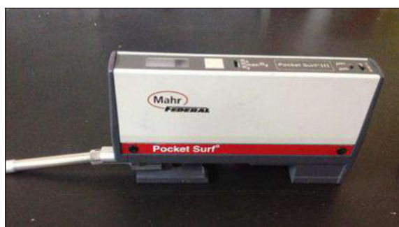
Figure 8. Surface profilometer used for surface roughness (Ra) measurement
