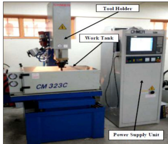
Figure 6. EDM machine used in the PMEDM experiments
