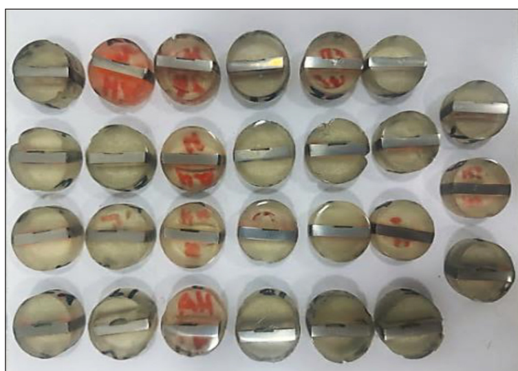
Figure 10. Metallographic preparation of Ti-6Al-4V specimens for recast layer thickness measurement
