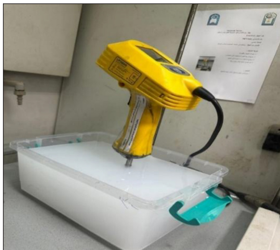
Figure 5. Ultrasonic probe homogenizer (sonicator) used for dispersing ceramic nano-powders in the dielectric fluid prior to the PMEDM experiments
