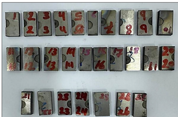
Figure 9. Sectioning of EDM specimens using wire electrical discharge machining (Wire-EDM)
