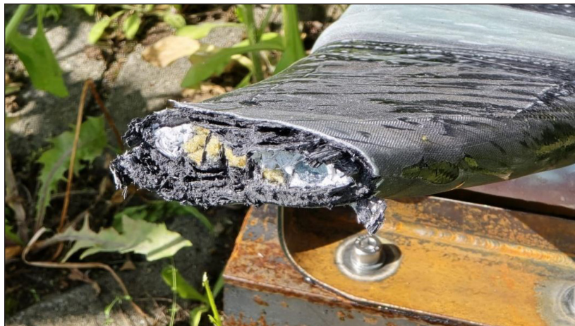
Figure 12. Close-up view of the landing gear fracture zone after the component-level destructive test
