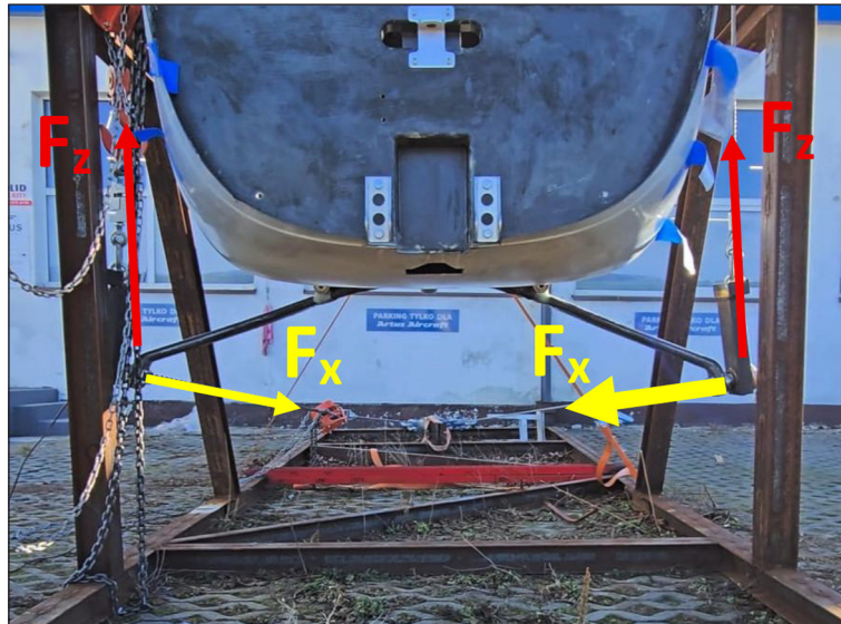
Figure 9. Landing gear installed in the representative aircraft fuselage structure during the airframe-level strength test. The fuselage was attached to the steel test frame through the wing attachment fittings, with an additional restraint connected to the tail boom to limit the pitching moment transferred through the wing attachment points. The arrows indicate the longitudinal [ F_x ] and vertical [ F_z ] force components applied simultaneously at the wheel.
