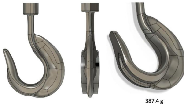
Figure 14. Final geometry obtained from generative design
