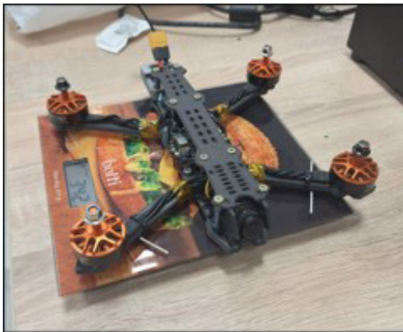
Figure 9. Assembled quadcopter structure
