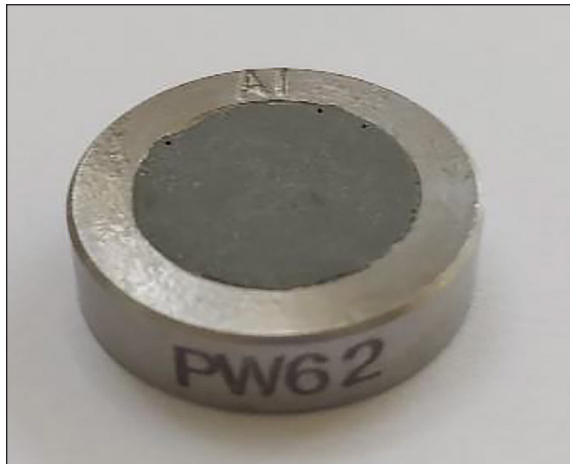
Figure 3. The stress free powder sample A1, PW62
