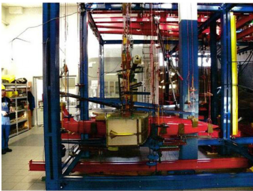
Figure 15. OCP airframe during testing and loading system
