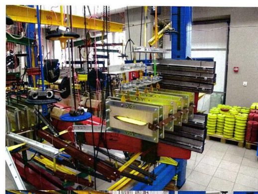
Figure 15. OCP airframe during testing and loading system
