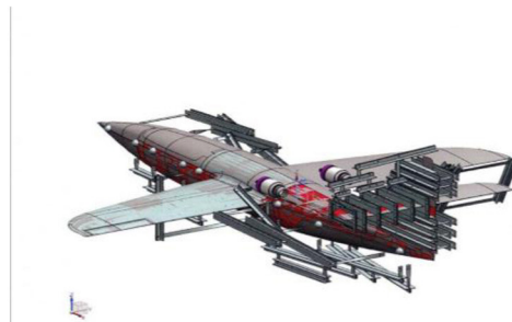
Figure 16. The OCP during fuselage and tail tests (horizontal and vertical) and the loading system (CAD model)
