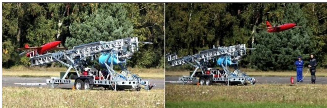
Figure 2. Launch of the OCP from a pneumatic launcher
