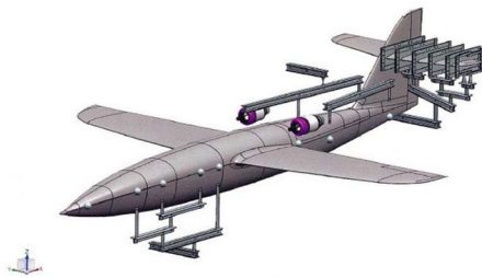
Figure 16. The OCP during fuselage and tail tests (horizontal and vertical) and the loading system (CAD model)
