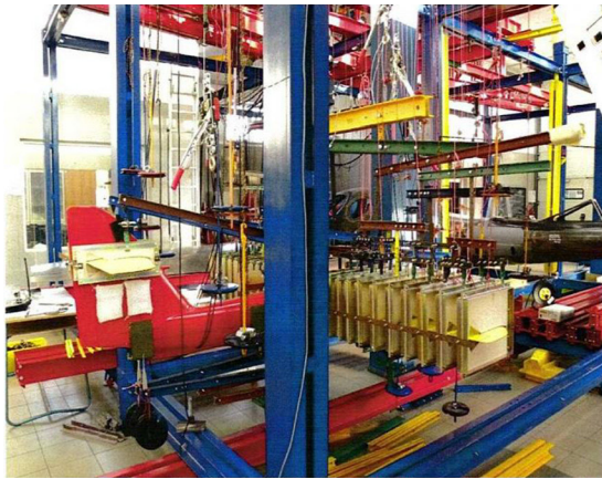
Figure 15. OCP airframe during testing and loading system
