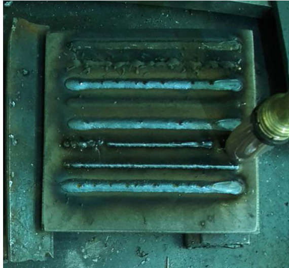
Figure 3. Example S355 steel plate after the MAG surfacing experiment, showing eight deposited weld beads produced under different process parameters.
