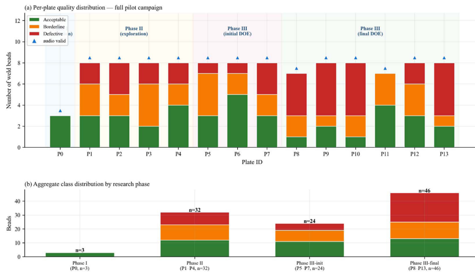
Figure 4. Overview of the experimental campaign. (a) Per-plate distribution of weld bead quality labels across the experimental phases. (b) Aggregate sample counts per phase
