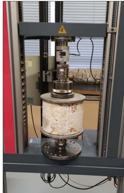
Figure 4. Test of 10% deformation of the mycelium biocomposite material [44]
