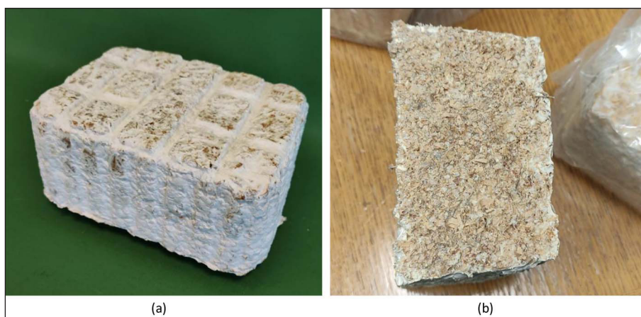
Figure 1. Mycelium-bound biocomposite block subjected to testing (a), cross-section of the tested block (b) [44]
