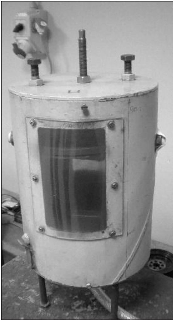
Figure 3. General view of the pneumatic shot peening station
