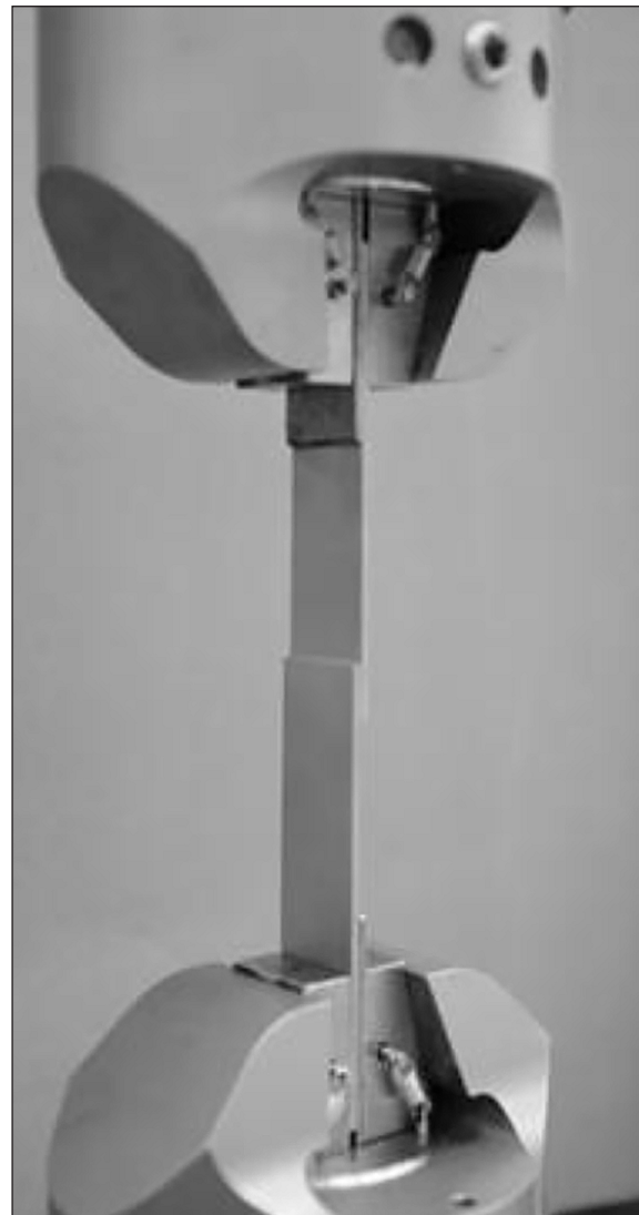
Figure 4. Method of mounting samples for strength tests
