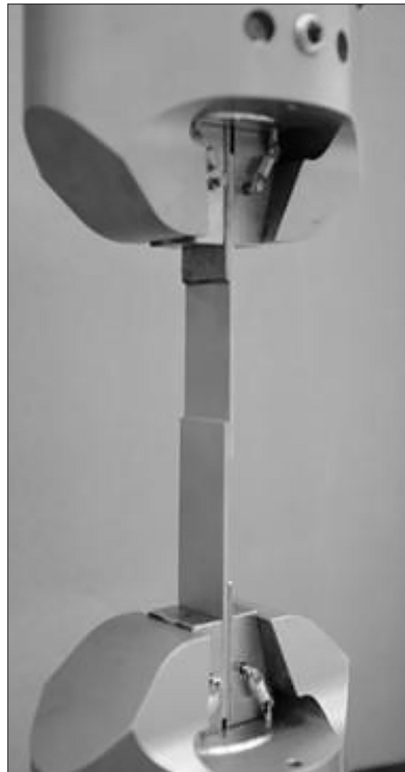
Figure 4. Method of mounting samples for strength tests
