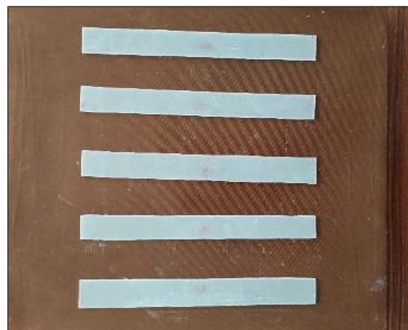
Figure 3. Fabricated unidirectional glass/epoxy laminates after trimming to tensile test dimensions
