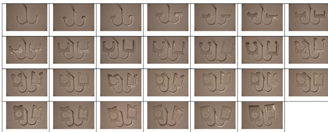
Figure 19. Short injections at 0.025 second intervals for PP + 1.5% ba, (27 short shots total)
