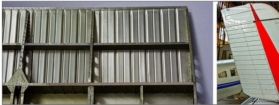
Figure 3. Corrugated stiffening of control surfaces
