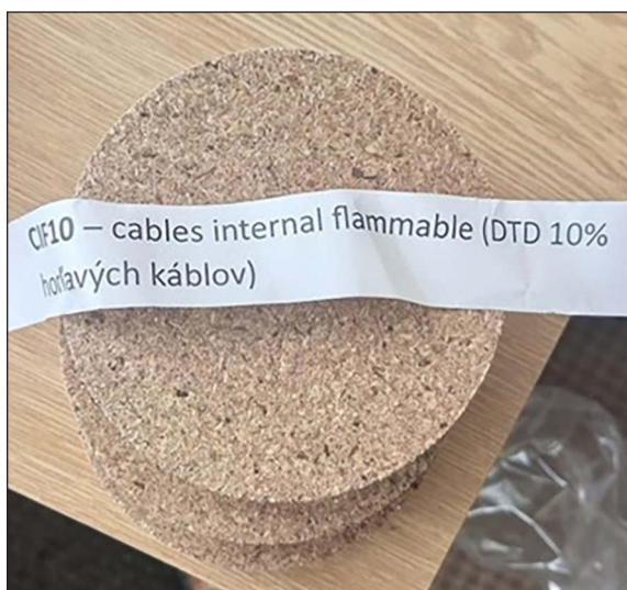
Figure 2. View of sample specimens for acoustic testing
