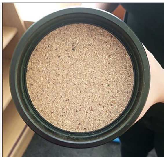
Figure 2. View of sample specimens for acoustic testing
