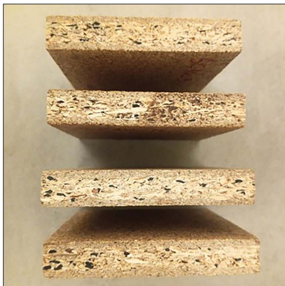
Figure 1. Macroscopic view of the cross-section of selected samples
