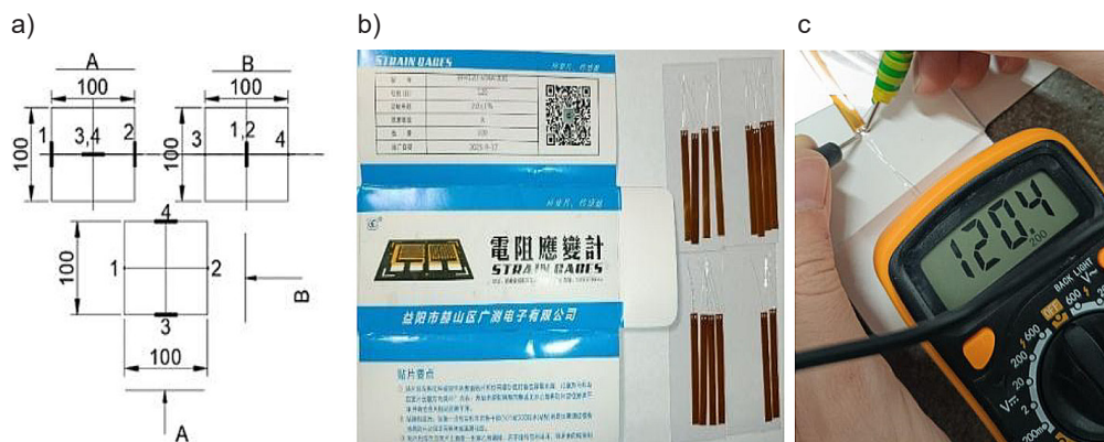
Figure 5. a) Scheme for gluing strain gauges onto cube samples, b) BX120-50AA 120-50AA Gauge concrete, c) PM830B high accuracy digital multimeter
