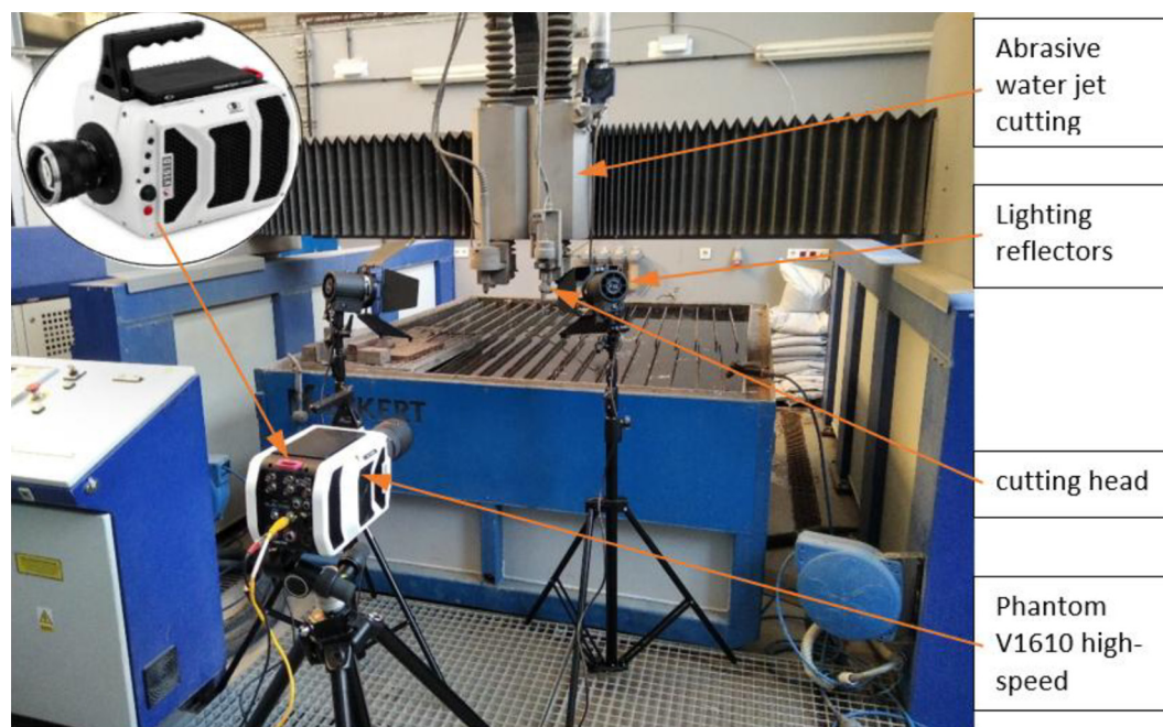
Figure 1. Experimental setup used in the study, including the Eckert Combo abrasive water jet cutting machine and the rapid-event recording system with a high-speed camera Phantom V1610 and lighting system
