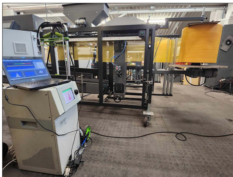
Figure 1. View of the slitter (cutting module) with measurement equipment in operation
