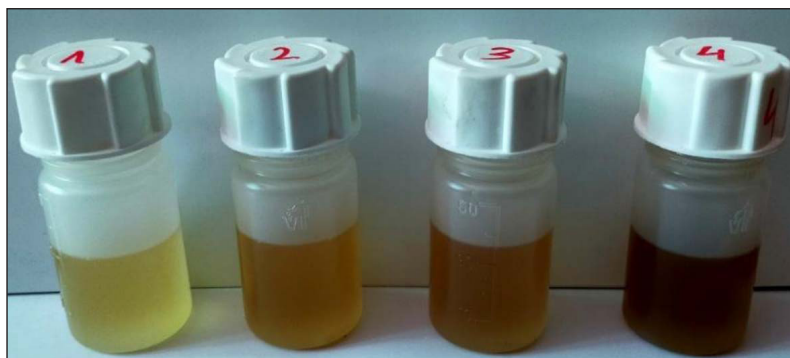
Figure 3. View of tested hydraulic oil samples (1 – fresh oil, 2 – oil after 200 hours of operation, 3 – oil after 400 hours of operation, 4 – oil after 600 hours of operation)
