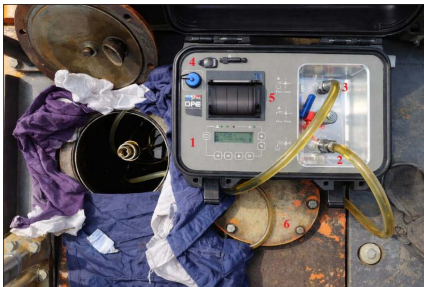
Figure 2. Method of conducting tests directly on the excavator: 1 – top side with control panel, 2 – suction line internal pump, 3 – drainage of oil into the tank, 4 – charger connection, 5 – printer, 6 – excavator oil tank
