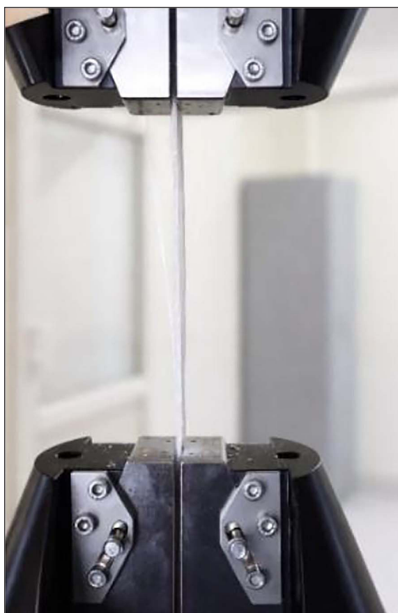
Figure 3. Fatigue testing setup for tension–tension fatigue loading
