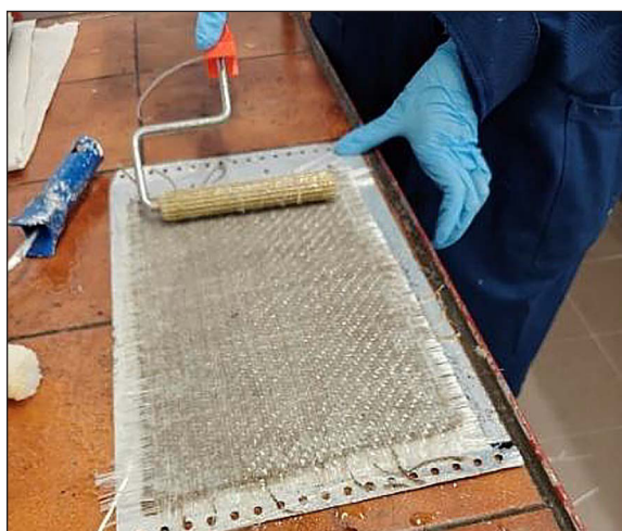
Figure 2. Application of epoxy resin in the hybrid composite
