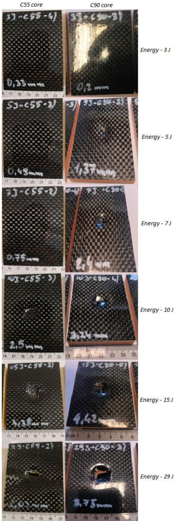
Figure 7. Examples of sample damage resulting from puncture resistance testing
