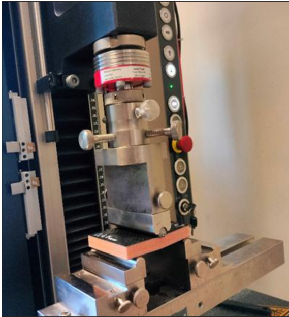
Figure 8. A sample during flexural strength test
