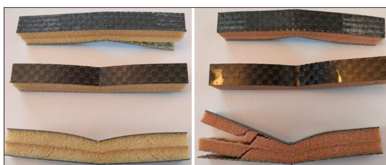
Figure 4. Fractured samples after surface impact strength testing: (a) the samples with a C55 core; (b) the samples with a C90 core
