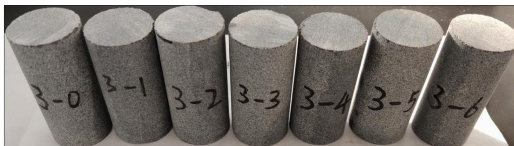
Figure 1. Prepared sandstone specimens
