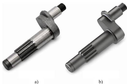
Figure 1. Crankshaft: (a) actual component, (b) 3Dmodel
