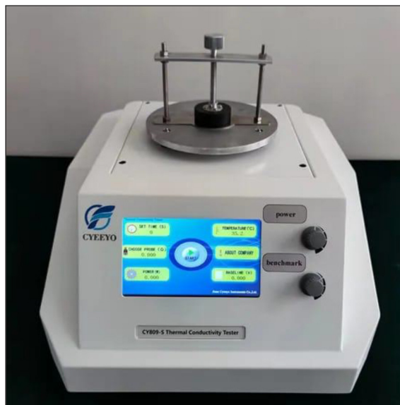
Figure 2. Hot-Disk device with specimen
