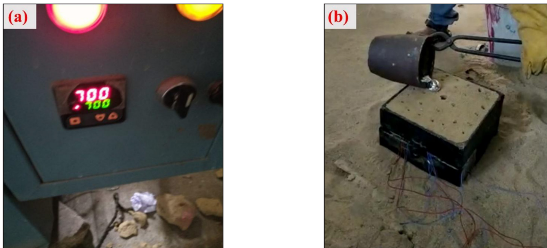
Figure 1. Photograph of (a) pouring temperature used, (b) pouring of molten metal
