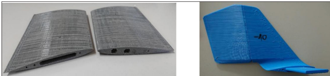
Figure 4. Horizontal and vertical stabilisers [12]
