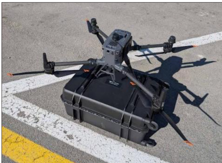
Figure 1. The UAV with Septentrio Mosaic-X5 receiver before flight experiment
