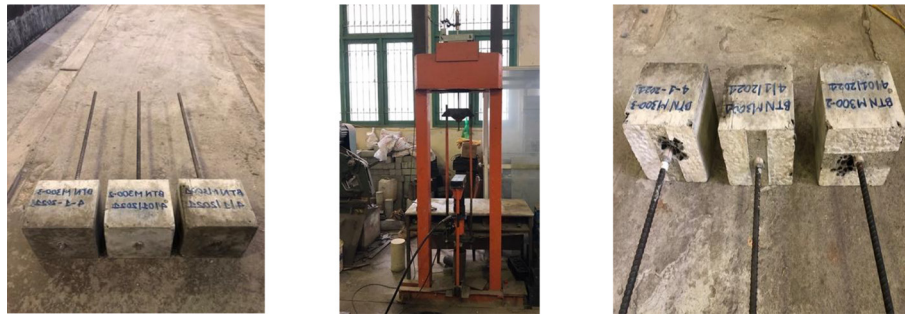
Figure 4. Test specimens, pull-out test setup, and failed specimens
