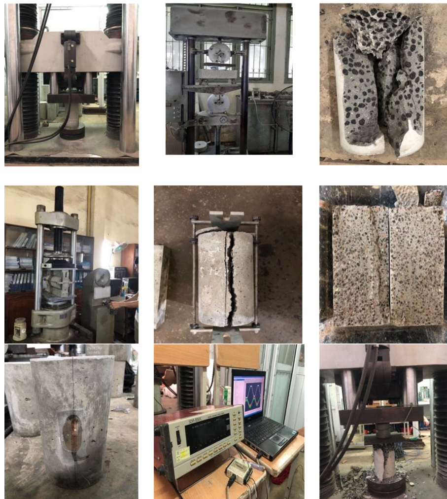
Figure 3. Test specimens, testing equipment, and failed specimens from the mechanical and physical property tests of recycled lightweight aggregate concrete
