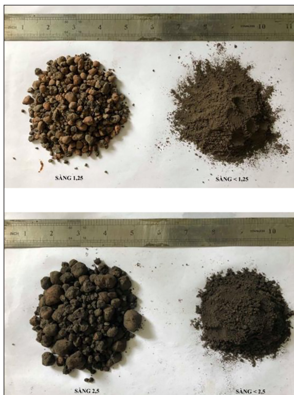
Figure 2. S2 and S3 aggregate samples after the crushing test and sieving through different sieve sizes
