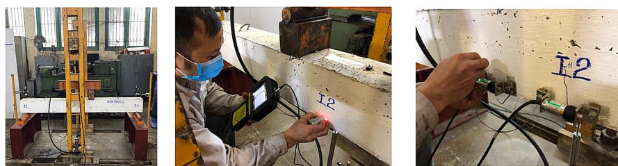
Figure 5. Four-point bending test setup and instrumentation layout
