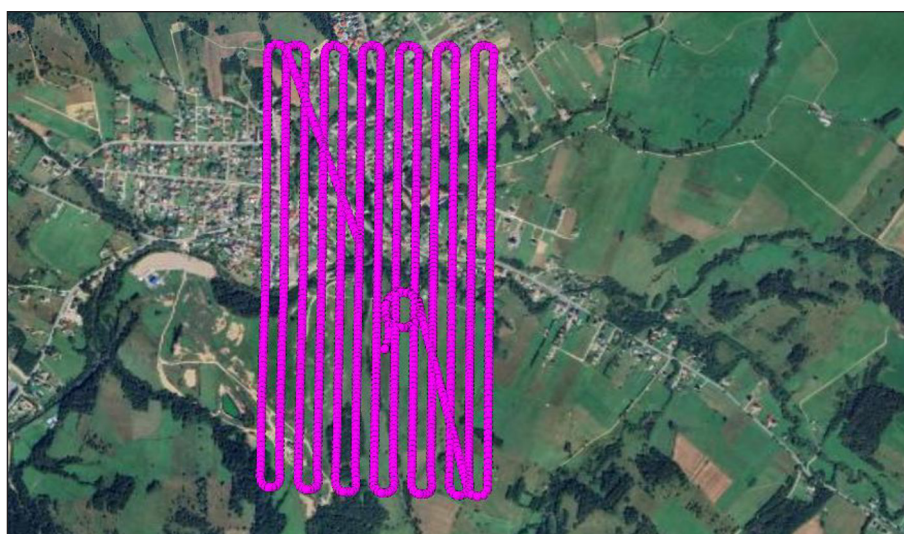
Figure 4. The flight trajectory of UAV [74]
