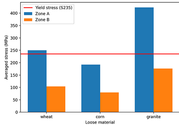
Figure 8. Changes in average stresses in different areas of a perforated plate for different loose materials ( a = 1 mm, s = 0.6 mm, k = 9 )
