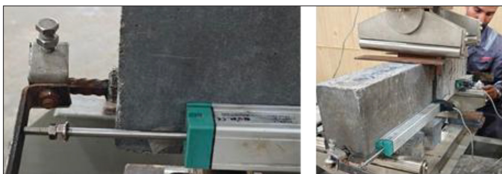
Figure 7. LVDTs installation on both sides
