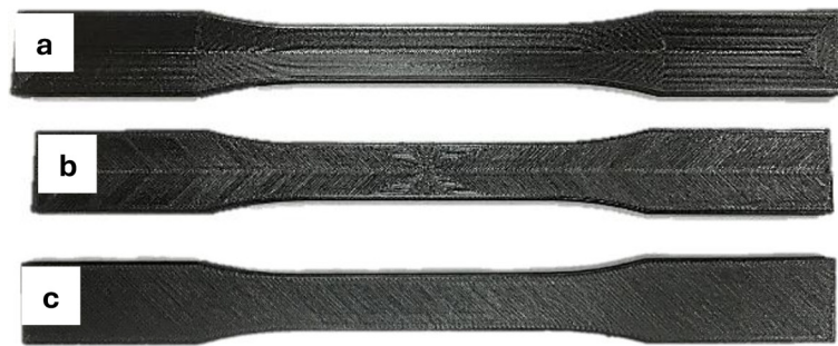
Figure 7. ASTM D38 Specimen. (a) Concentric, (b) Octagram spiral, (c) Rectilinear
