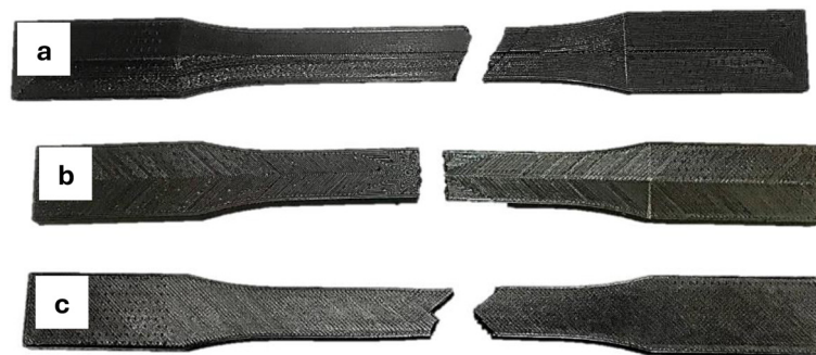
Figure 8. ASTM D638 Specimen after Tensile test. (a) Concentric, (b) Octagram spiral, (c) Rectilinear
