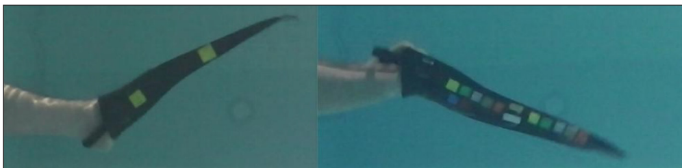
Figure 3. Fins with coloured markers during the pool tests
