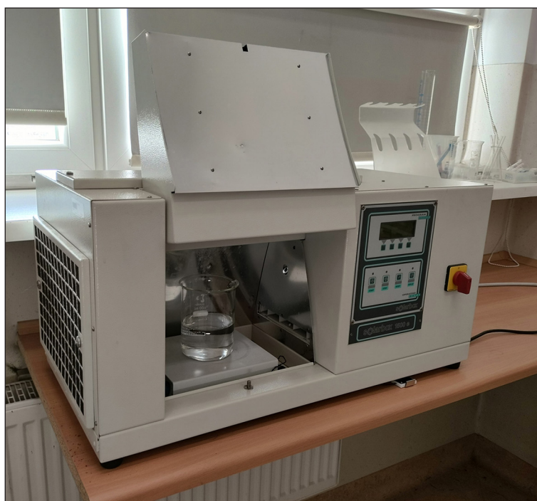
Figure 2. Solar simulator (Solarbox 1500e)
