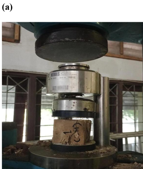
Figure 7. (a) Compressive strength test and (b) Flexural strength test
