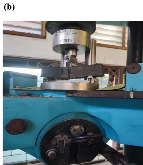
Figure 7. (a) Compressive strength test and (b) Flexural strength test
