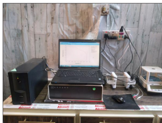
Figure 2. The potentiostat instrument used for the corrosion test
