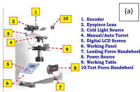
Figure 7. (a) Vickers hardness tester setup. (b) specimen size and shape
