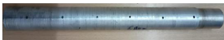
Figure 15. Prepared Specimens with Thermocouple holes to perform temperature measurement throughout the specimens
