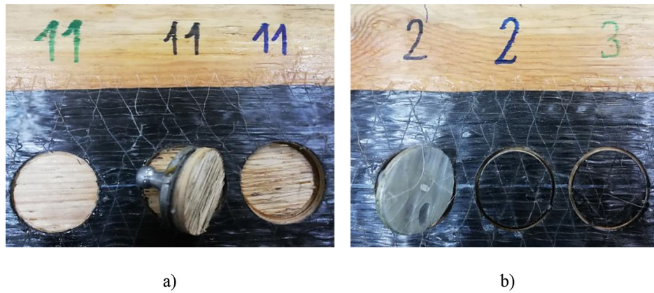
Figure 12. Graphical presentation of the following type of damage: a) „a” - visible layers of detached wood and damage to the wooden beam, b) „d” - A 1 mm thick layer of glue is visible on the disc surface, indicating a lack of cooperation between the disc and the CFRP composite
