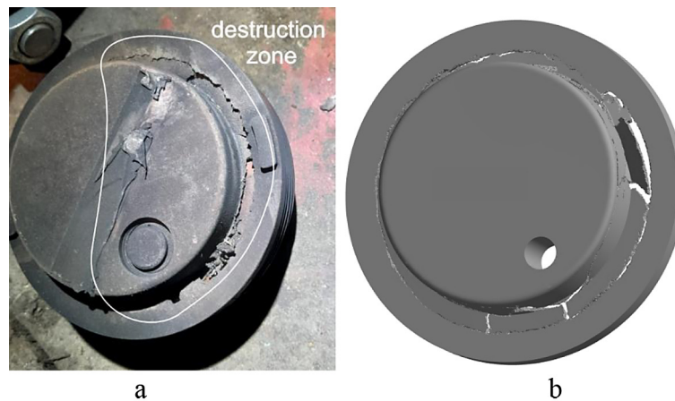
Figure 13. Destruction of the landmine fuze: (a) experiment; (b) numerical modelling
