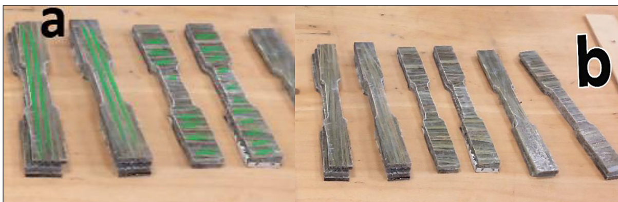
Figure 4. a. Composite plate: Natural fiber composite oriented horizontally, b. Test specimens: Various cross-sectional shapes arranged vertically for evaluation
