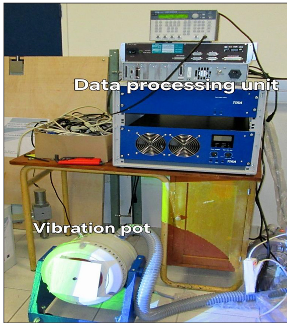
Figure 5. Vibration pot and data processing unit: Equipment setup for vibration testing and data analysis
