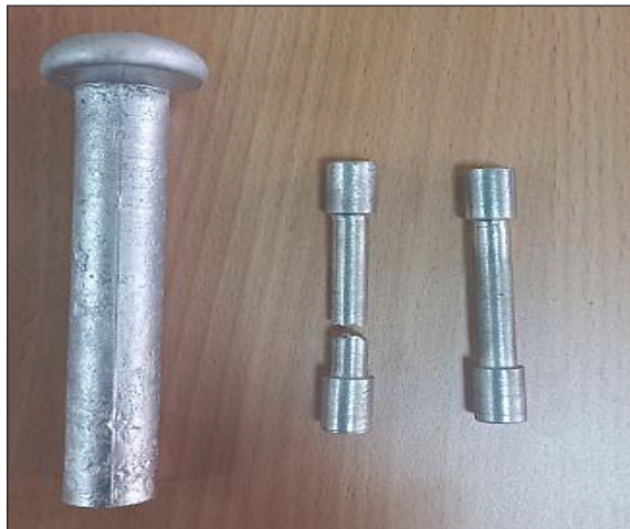
Figure 3. The sample after casting and the samples before and after tensile testing
