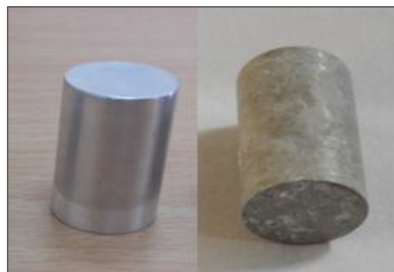
Figure 4. Corrosion samples before and after test 4%wt
